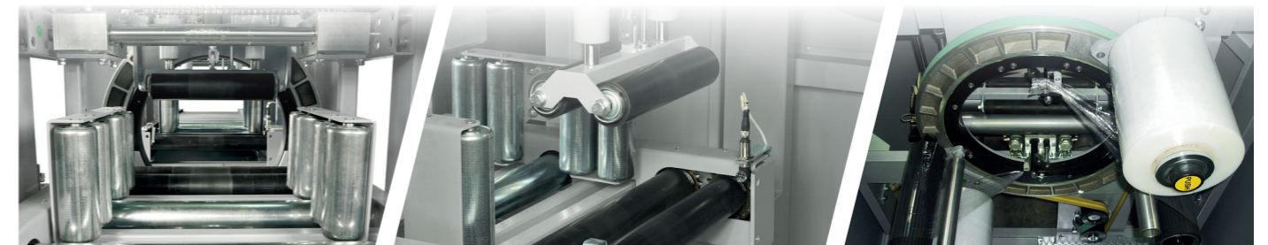
GUIDE LATERALI A RULLI IN ENTRATA E USCITA / INCOMING AND OUTGOING SIDE ROLLER GUIDES
