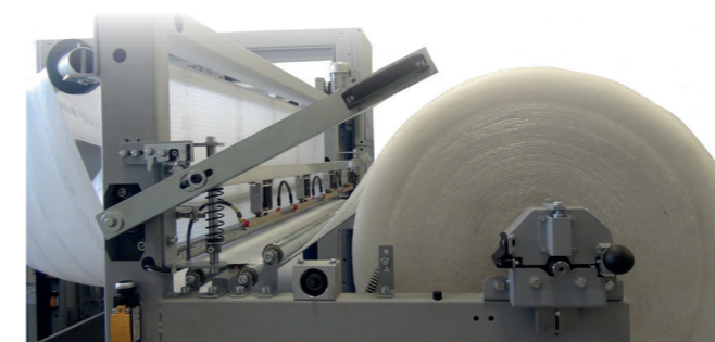
CAMBIO BOBINA FACILITATO (OPT.) GRAZIE AL SALDATORE MANUALE. Include allarme bobina quasi finita. EASY REEL CHANGE (OPT.), THANKS TO THE MANUAL WELDER. It includes almost finished reel alarm.
