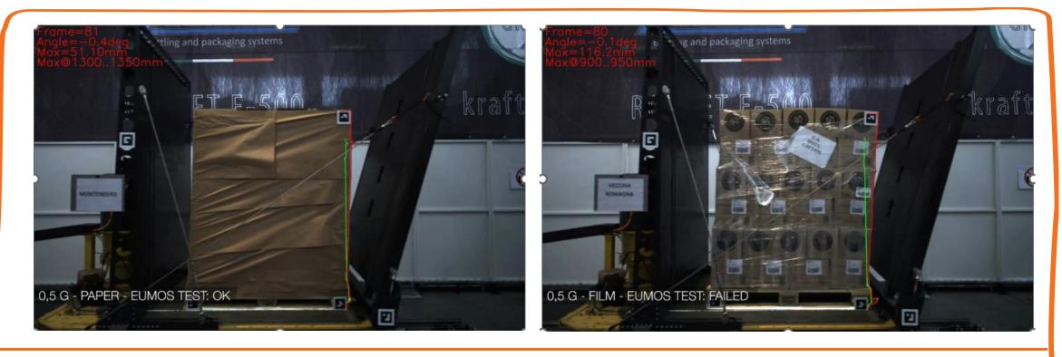
The pallet wrapped in Stretchwrap has 30% less vertical deformation vs a pallet wrapped in stretch film.
